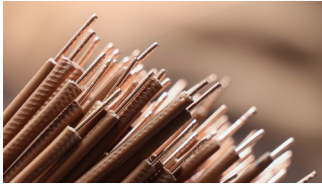
Laser Hairpin Stripping: Clean, repeatable laser stripping for high-volume e-mobility production.
